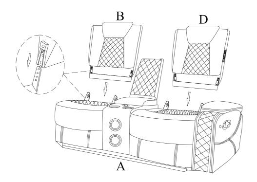
STEP 3: Insert the right wing (E) to the backrest (D) and make sure it is secured in position .
