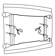
Step 2: Please align and insert the metal bracket (F) on the backrest onto the metal bracket (M) of the seat. Please make sure the metal brackets (F) and (M) are inserted all the way and secured into position.
