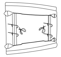
Step 2: Please align and insert the metal bracket(F) on the backrest onto the metal bracket (M) of the seat. Please make sure the metal brackets (F) and (M) are inserted all the way and secured into position.
