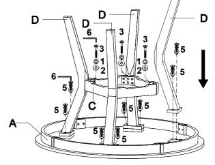
Don't tighten the bolts untill last step
