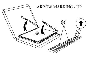
STEP 2: Align & fasten mirror support (B) to the back of mirror (A) using short JCBC bolt(1), spring washer (3) & flat washer (4). DO NOT FULLY TIGHTEN AT THIS STEP.
